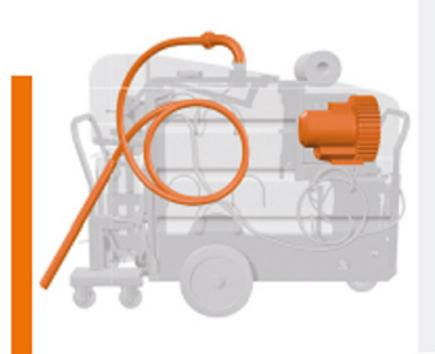
High-suction pump for extraction of process medium to be cleaned.
